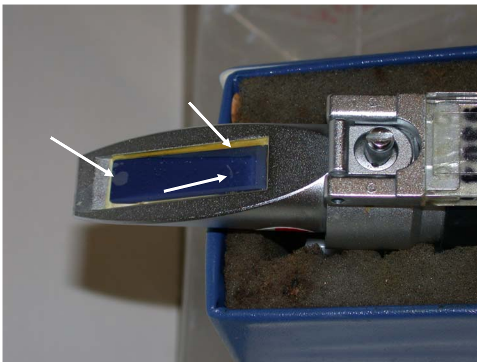
Figure 9. Poorly maintained refractometer with a damaged prism. Scratches, separations, and detached prism noted by arrows.
