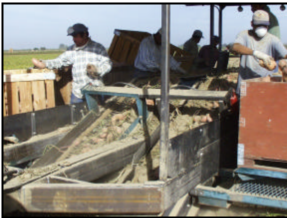
Two-row diggers have arrived to California. They're big and need a lot of room to turn, but offer considerable improvements in labor and tractor efficiency.
